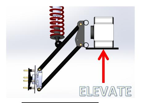
**STEP ONE:** First thing that needs to be done is to get the end you are measuring elevated. This gets you to the largest angle and distance your vehicle will need when in operation.
