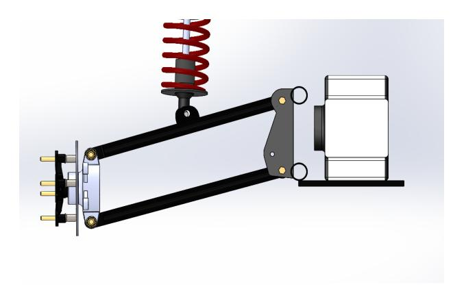
**STEP FIVE:** Once the vehicle is back on the ground you will need to take the same measurements. The reason being to get your compressed length. This is necessary to give your vehicle the best functionality at performance.
